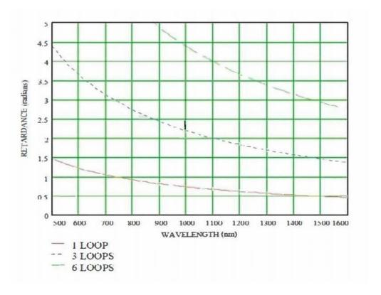
Relationship between single-loop delay and wavelength, number of loops in polarization controller.(Test unit: fiber loop diameter 40mm, fiber cladding diameter 900µm) For example: Polarization controller fiebr loop fixed diameter of 40 mm, the cladding diameter of 900µm of tight-sheathed fiber around in the ghost.
